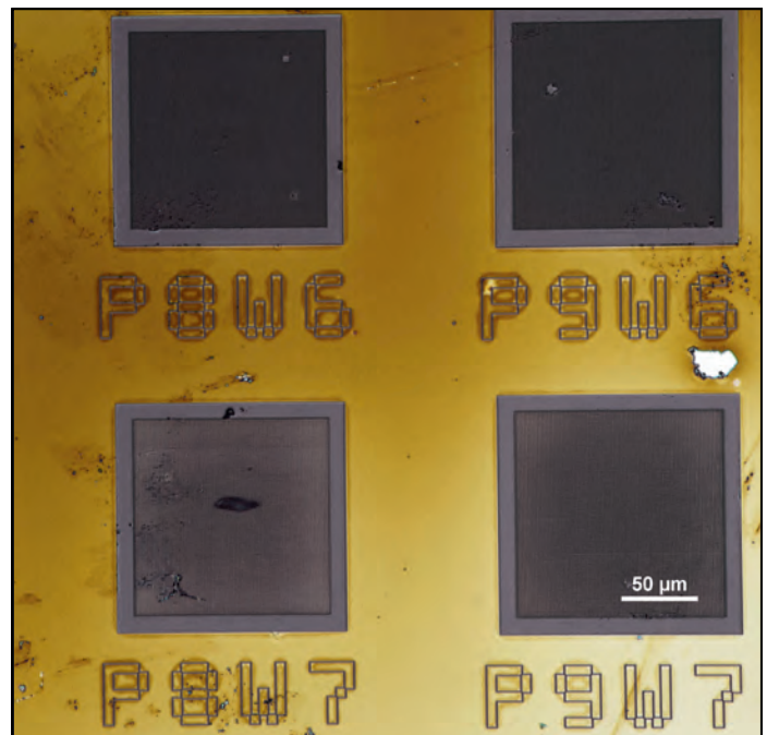
Optical microscope images of fabricated metasurfaces with a size reference scale of 50 microns. © Graph created by the student researcher using Adobe Illustrator, 2025. Image collected using optical microscopes and SEMs in MIT. Nano.
