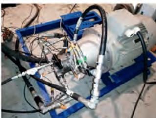
(a) HPU model with tested pump
