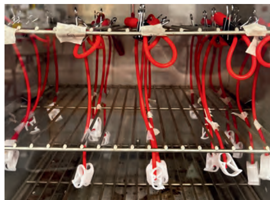
Figure 2: The clogged J tubes placed in the incubator; vertically oriented. Photo taken by student researcher, 2026
